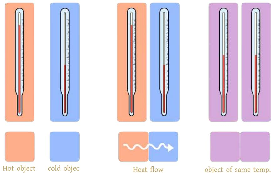
When a hot object is brought into contact with a cold object, heat will flow from the hot object to the cold object until the temperature is equal.
